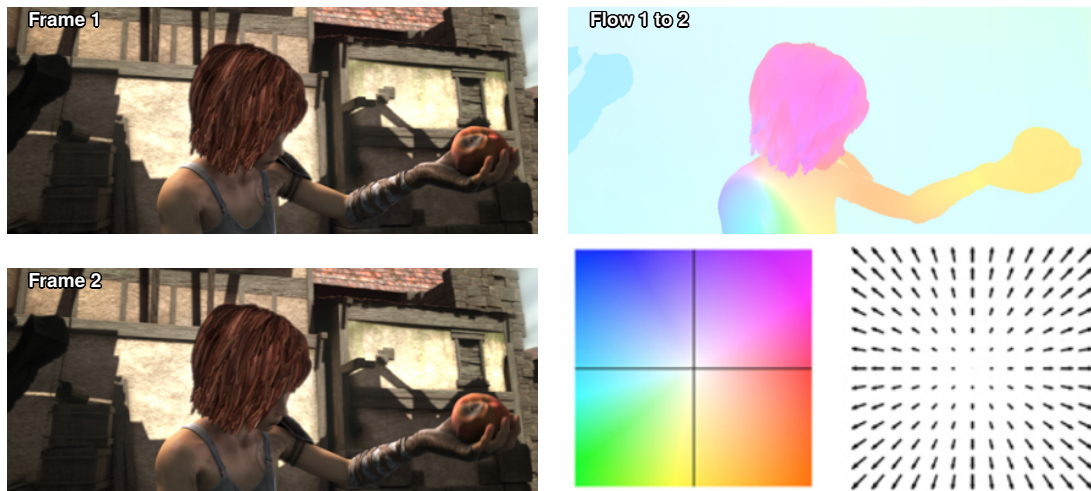
Figure 2.7: Visualizing inputs to optical flow prediction tasks and the ground truth motion map in MPI Sintel dataset [15].
