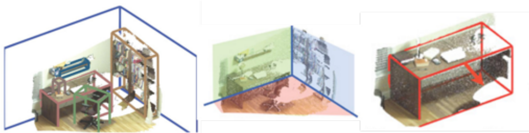
Figure 2.5: Visualizing 3D cuboid annotations for objects and room layouts in SUN RGB-D dataset [118].
