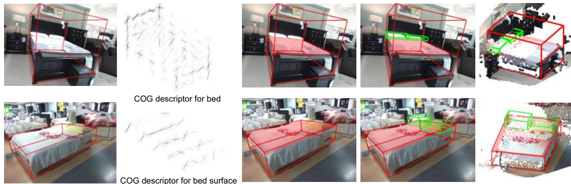
Figure 3.9: A visualization of 3D object detection system for beds and pillows using latent support surfaces. Given input RGB-D images, we use our learned COG descriptor [99] to localize 3D objects and infer latent support surfaces (shaded) for 3D proposals of beds (red). Then we search for pillows (green) that lie on top of the inferred support surfaces.
